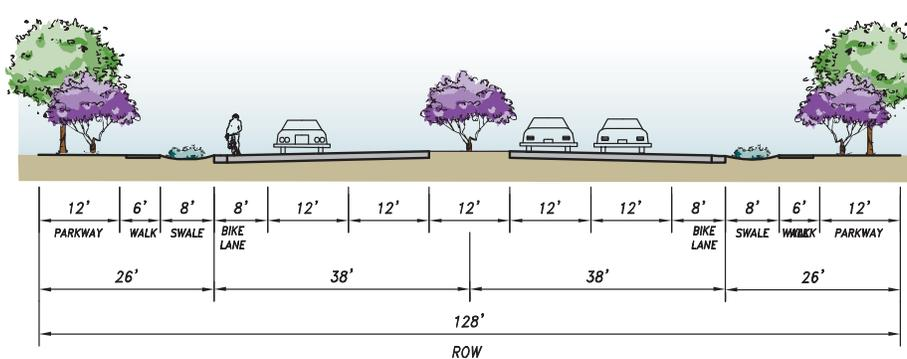
Figure M-2: Proposed Roadway Network Street Cross Sections (continued)
